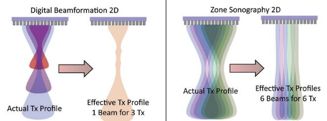
Therefore, transmit beam density is no longer determined by the round-trip beam as is generally the case with conventional imaging.
